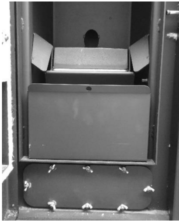
Figure 54 - Cleaning the interior of the unit
