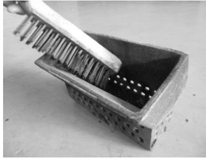
Figure 53 - Cleaning the burning basket
