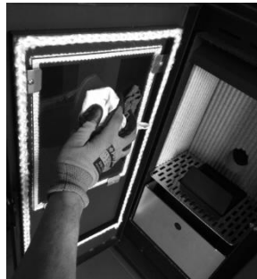
Figure 61 - Cleaning of the glass: a) moisten a soft cloth with liquid; b) clean the glass with the cloth
