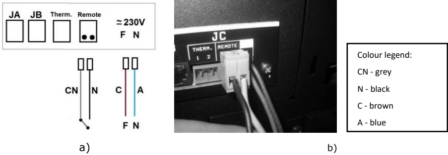
Figure 44 - Connection of the wireless remote control
