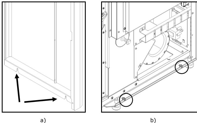
Figure 96 – Assembly of the covers
