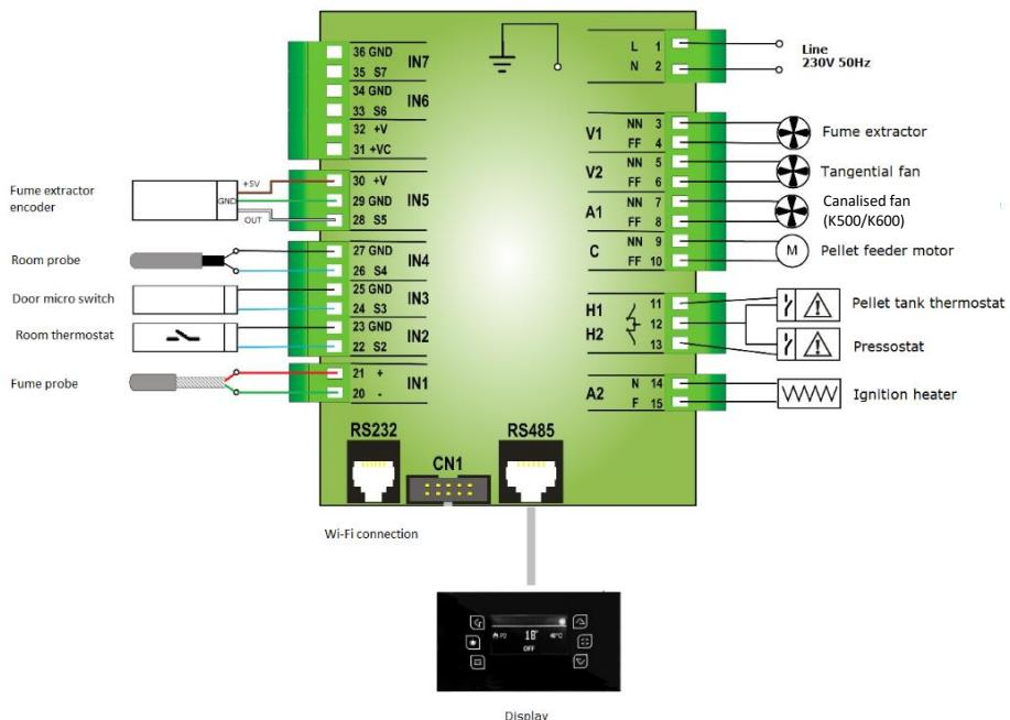
Figure 154 – Electrical diagram (Columbus electronics)
