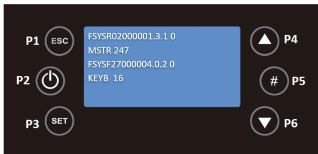
To return to the Display menu, press P1. Pressing this key twice will display the Settings, Display, Service and System menus.
