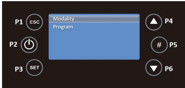
By selecting Mode with the P3 key you can select which Chrono mode you want. Use the P4 and P6 keys to select between Daily, Weekly and Weekend, use the P2 key to activate/deactivate the choice and P3 to save the changes.
