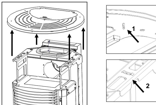
Figure 74 – Removing the top cover
