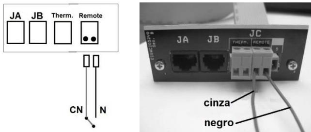
Figure 149 – Connecting the wired remote control
