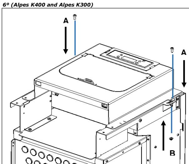
Figure 56 - Fixing the top of the equipment frame
