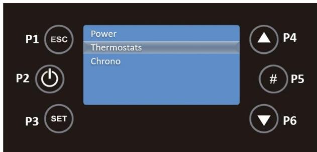
In this menu, select the submenu Room, using the P3 key.
