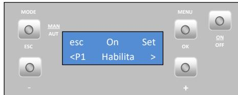
To set the **starting time** for Programme P1, press "set". The display starts to flash. Press the "+" or "-" key to select the time and then press "ok" to confirm. Press the "+" key to go to the "P1 A. Stop" menu.
