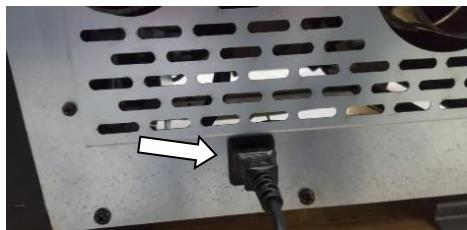
Figure 8 - Electric power plug
