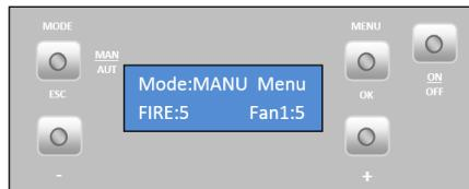
**FAN 1 (built-in fan):** In both AUTO and MANU modes it is possible to vary the fan speed by pressing the "+" button for 3 seconds. You can choose values from 1 to 5 and "A" where the value 1 corresponds to the lower speed and the value 5 to the higher speed of the fan, it is **RECOMMENDED** to use the value "**A**" means **automatic**.
