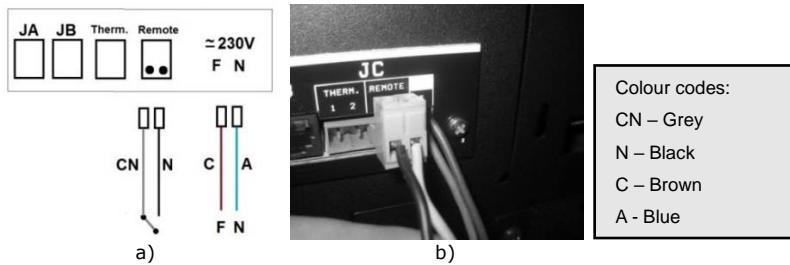
Figure 148 – Connecting the wireless remote control
