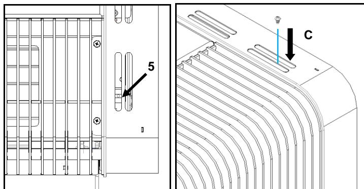
**Figure 90 – Assembly of the Aspen covers**
