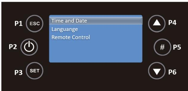
In the Date and Time menu, select Time, with the P4 and P6 keys, and press the P3 key, the time will appear in editable mode, flashing, with P4 and P6 select the correct time and press P3 to validate.
