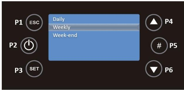
You must press P3 and this option will be in editable mode, flashing. Press P4 and P6 to select the desired time and then use the P3 key to save. Repeat this process for the time at which the unit is to shut down, using P4 and P6. Finally, activate the interval by pressing P5, and a check mark will appear to the right of the interval.
