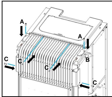
Figure 88 – Front grille tightening
