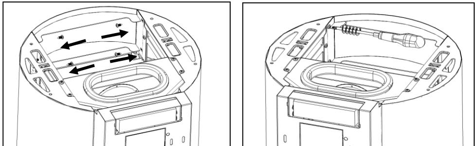
Figure 81 – Attachment of the cover to the front
