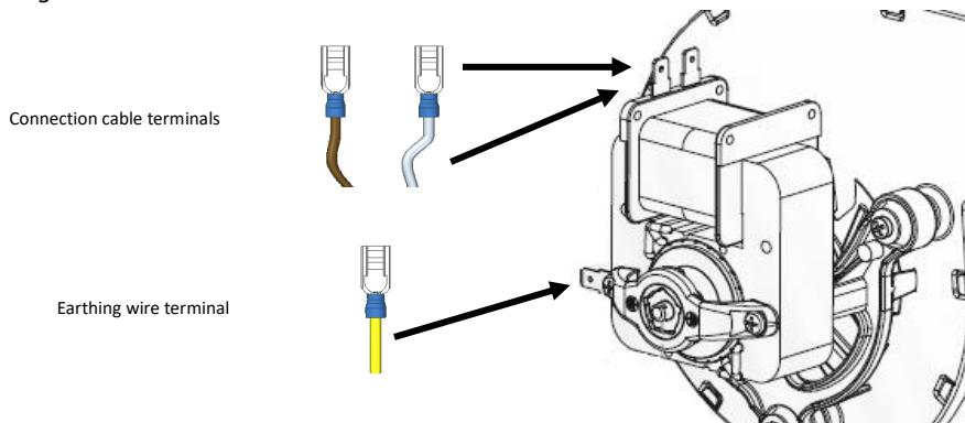
**Figure 118 – Connecting the cables to the ventilator**
