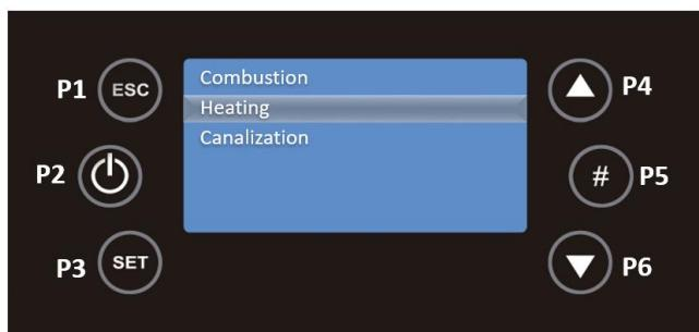
With the P4 and P6 keys, you can modify the system's combustion power. This submenu allows the system's heating power to be modified. It can be set in automatic or manual mode: in the second case, the user selects the power from 0 to 5.
