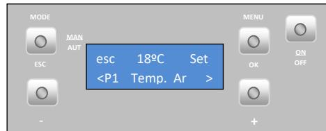
To set the **operating power level** (1 to 5) of Programme P1, press "Set". The display starts to flash. Press the "+" or "-" key to select the desired power level (1 to 5), and then "Ok" to confirm. Press the "+" key to go to the "P1 Dia" (P1 Day) menu.
