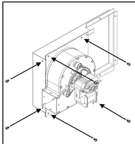
Figure 127 – Securing the support bracket to the ventilator
