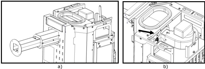
**Figure 114 – Fitting the air guide to the free-standing fire unit**
