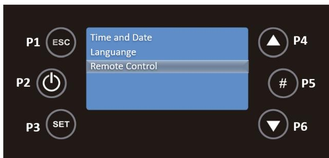
With the P4 and P6 keys you can activate or deactivate the Remote Control, pressing P3 to validate the option.
