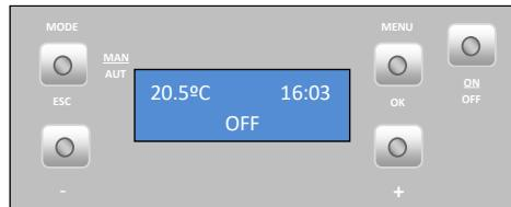
**Selecting the operating mode:** To select the operating mode, press the "Mode" key to select "Manu" for manual mode or "Auto" for automatic mode.
