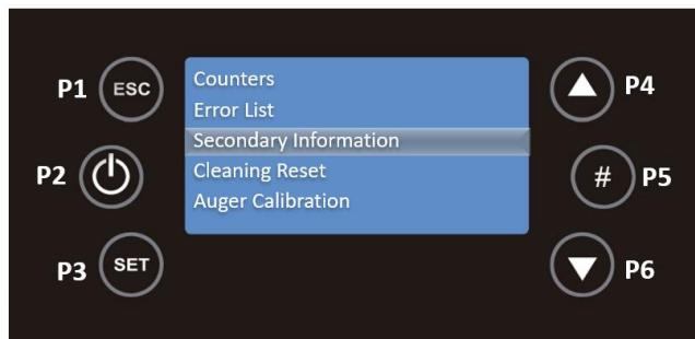
In this function you can check the product code, the status of the fan, the auger, the heating fan and the status of the outputs.
