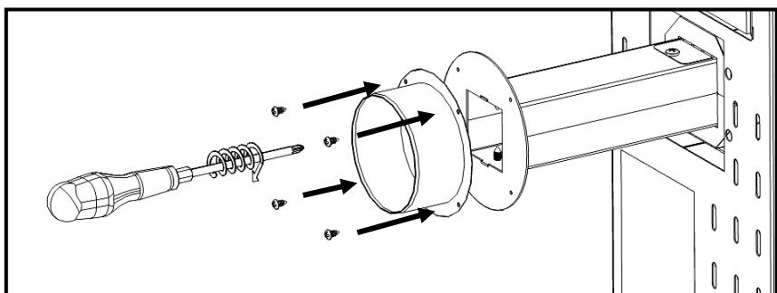
Figure 116 – Securing the air outlet duct to the free-standing fire unit
