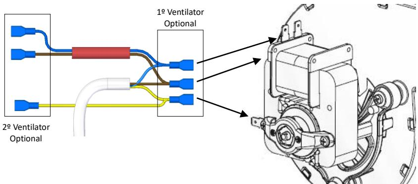
Figure 134 – Connecting the cables to the ventilator
