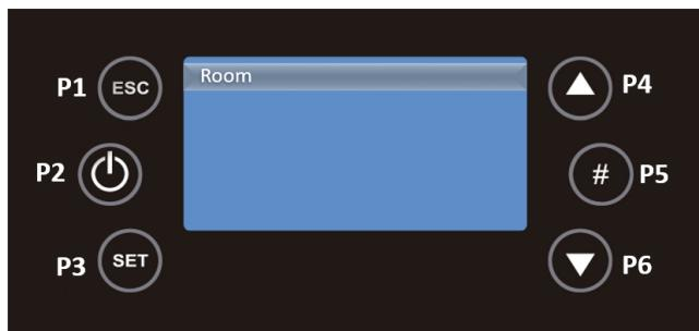
You can set the comfort target temperature between 10 and 40°C, with the P4 and P6 keys.
