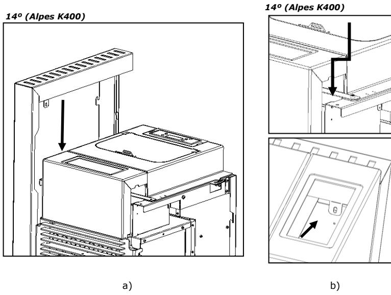
Figure 66 - Attach the tabs to the side frames
