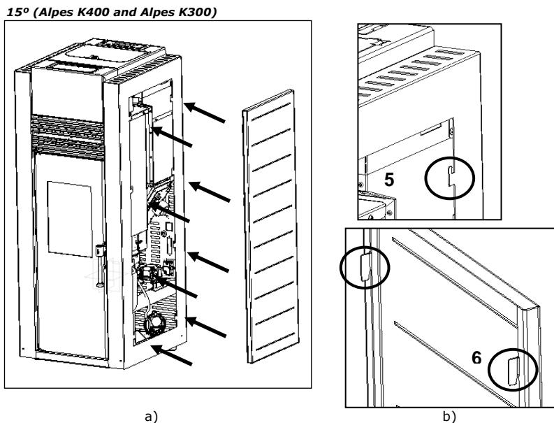
Figure 68 - Placement of the side cover panels
