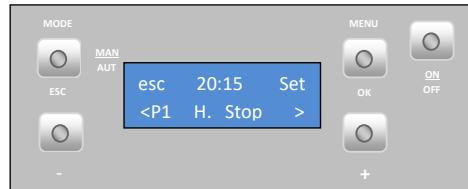
To set the **set point temperature** for Programme P1, press "Set". The display starts to flash. Press the "+" or "-" key to select the desired temperature, followed by "Ok" to confirm. Press the "+" key to go to the "P1 Temp. Água" (P1 Water Temp.) menu.
