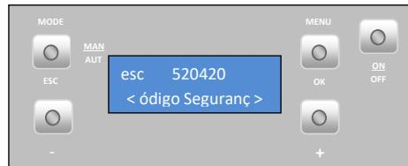
Software code / Display firmware. Press the "+" key to scroll to the "Código de Parâmetros" (Parameter Code) menu.
