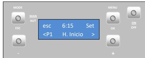
To set the **stopping time** for Programme P1, press "set". The display starts to flash. Press the "+" or "-" key to select the time and then press "ok" to confirm. Press the "+" key to go to the "P1 Temp. (P1 Air Temp.)" menu.
