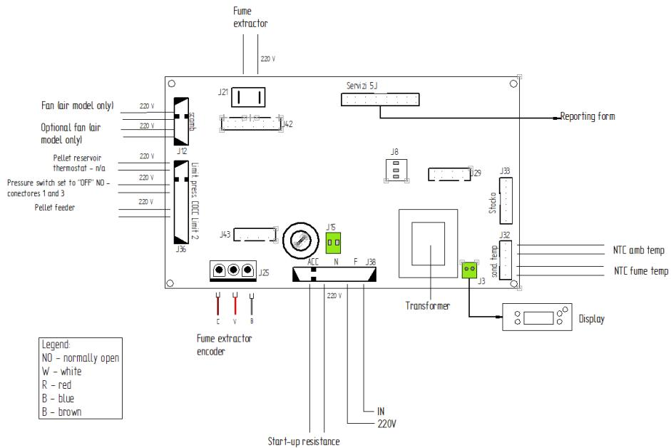
Figure 152 – Electrical diagram K100, K200, K500 and K600
