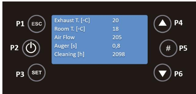
With the P4 and P6 keys you can scroll through the different variables. The values displayed are the values measured On-Line.
