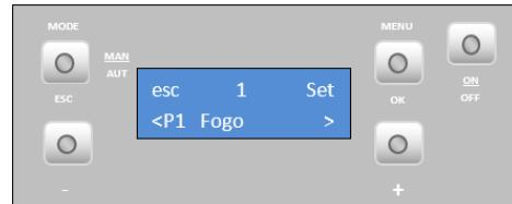
To select the **days of the week** that you want P1 Programme to run, press "set" and then select the day of the week using the "-" and "+" keys. Press "set". The display starts to flash. Select "On" or "Off" using the "-" and "+" keys. Press "ok" to confirm the selection. Press the "esc" key to go to the "P1 Dia" (P1 Day) menu. Press "esc" twice and then "+" to access the "Configurações" (Configuration) menu.
