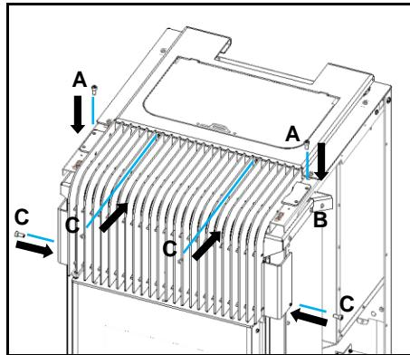
**Figure 103 – Front grille tightening**
