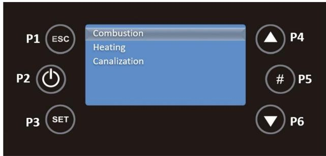
With the P4 and P6 keys you can modify the system's combustion power. It can be set in automatic or manual mode: in the first case, the system will choose the combustion power; in the second case, the user selects the power from 0 to 5.
