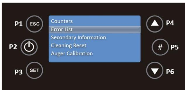
This submenu shows the last 10 errors that occurred, on each line the error code and the date and time when it occurred are displayed. To return to the Service menu press P1.
