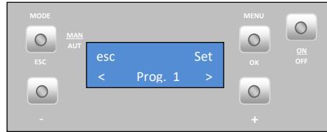
Press "Set" again and when the display starts to flash, press the "+" or "-" keys to select "On" or "Off". Press "ok" to confirm the selection. Press the "+" key to go to the "P1 A. Inicio" (P1 A. Start) menu.
