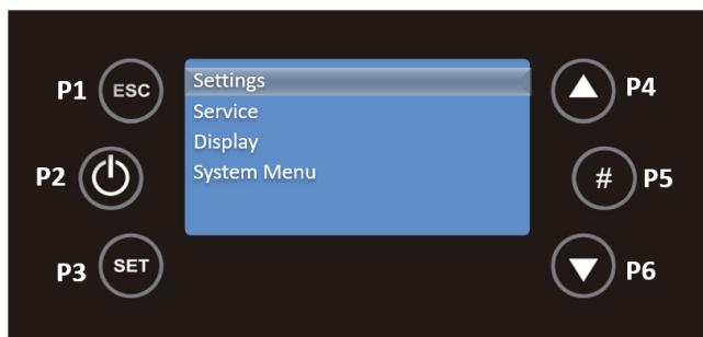
Use key P6 to select the submenu Remote Control and to validate the entry in this submenu the key P3.
