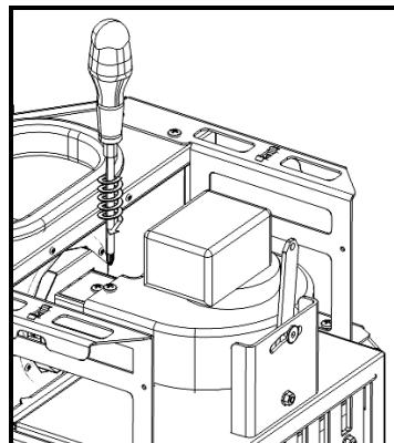
Figure 115 – Fitting the air guide to the free-standing fire unit
