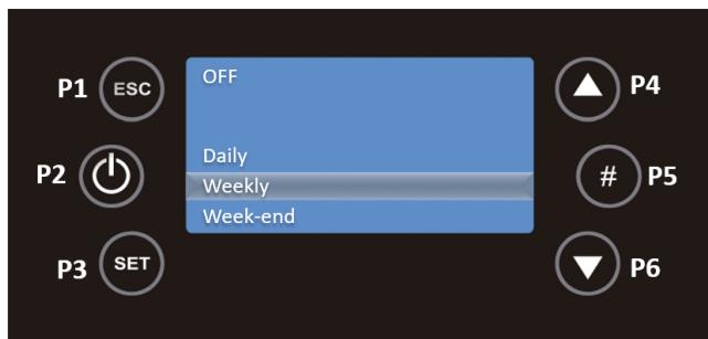
After activating the mode, the main screen will have Led **D**, **W** or **WE** active in the upper right corner.
