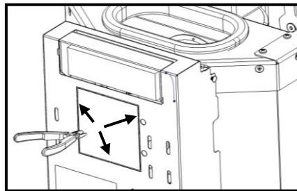
**Figure 113 – Removing the rear lid of the equipment**
