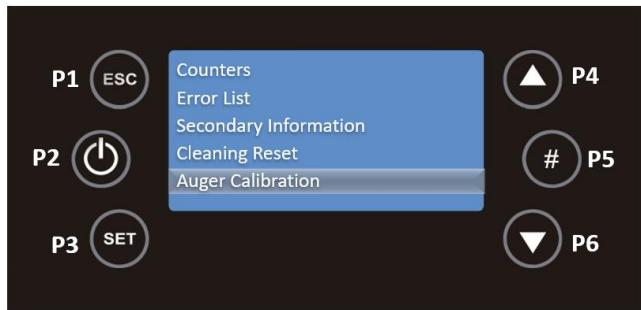
In this submenu with the keys P4 and P6 you can adjust the quantity of pellet to be fed, between -7 (-14%) and 7 (+14%). To return to the Service menu, press P1.
