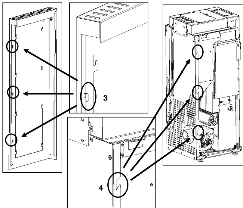
Figure 65 – Lateral attachment of lateral structures
