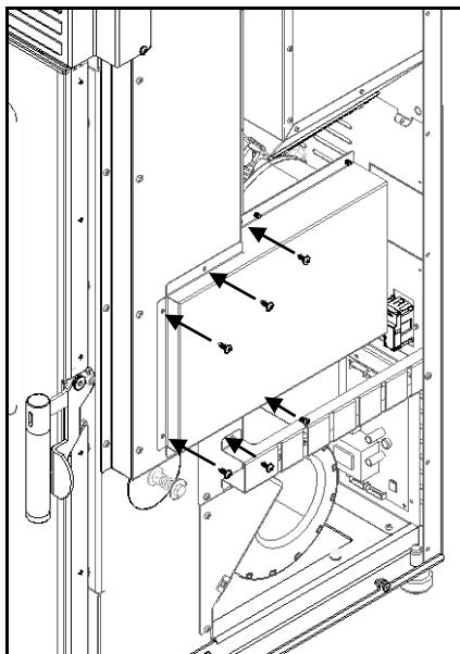
Figure 128 – Securing the ventilator to the unit
