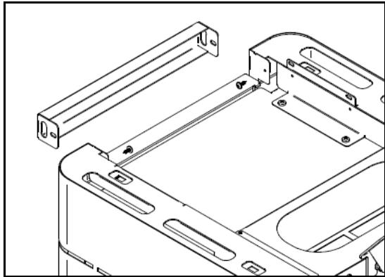
Figure 26 - Attaching the front on the K200 model
