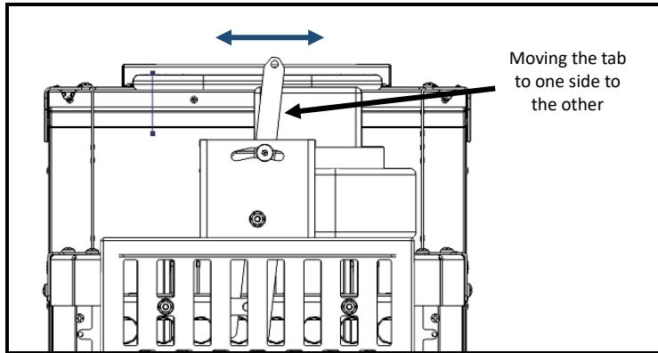
Figure 119 – Check the ductable air damper
