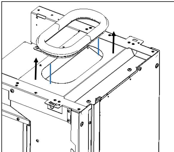
**Figure 52 - Removing the rubber seal on the equipment**
