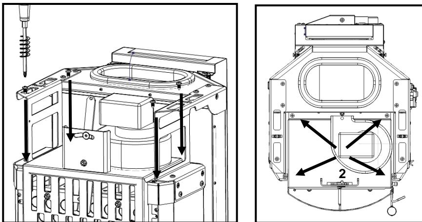
**Figure 112 – Fixing the ventilator to the equipment**
