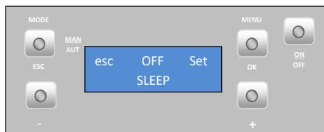
Press "set". The display starts to flash. Select the desired time using the "-" and "+" keys. After choosing the time, press "ok" to confirm. Press "esc" to return to the menu and "+" to go to the configuration menu.
