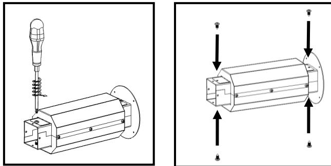
**Figure 122 – Reassembly of the thermal isolation**
