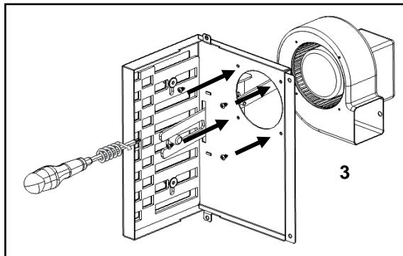
Figure 111 – Securing the support bracket to the ventilator
