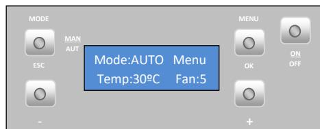
**"Auto" mode:** In this mode, the unit is turned on at maximum power until reaching a temperature 1°C above the selected temperature (set point temperature). After reaching the selected temperature, the unit switches to the minimum operating power. The set-point temperature can be set between 5 and 40°C by pressing the "-" key. The "+" key allows the user to set the fan speed between 1-5 or to automatic operation.
