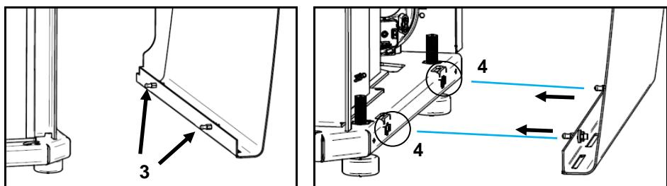
Figure 41 - Assembly of the Pine and Leaf covers
