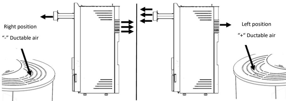
**Figure 123 – Adjusting the ductable air damper to "+" or "-"**
