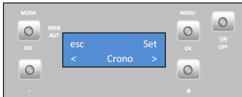
To **activate the Timer mode**, press “Set” - the display starts to flash. Press the “+” or “-” key to select “On” or “Off” and then “Ok” to confirm. Press the “+” key to scroll to the "Carga Perfil" (Profile Load) menu.
