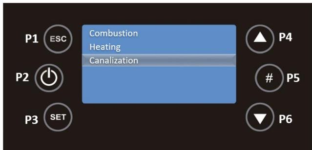
This submenu allows you to modify the power value of the canalization fan. It is only displayed if you select a heating system that includes a second heating fan. With the P4 and P6 keys it can be set in automatic or manual mode: in the second case, the user selects the power from 0 to 5.
