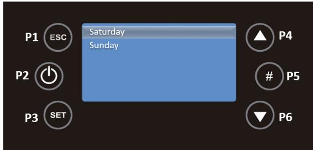
You must press P3 and this option will be in editable mode, flashing. Press P4 and P6 to select the desired time and then use the P3 key to save. Repeat this process for the time at which the unit is to shut down, using P4 and P6. Finally, activate the interval by pressing P5, and a check mark will appear to the right of the interval.
