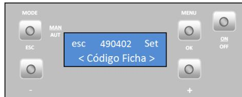
Software code / Security firmware. Press the "+" key to scroll to the "Código Display" (Display Code) menu.
