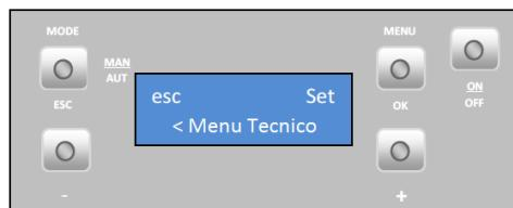
Press "Ok"; the letter "A" starts to flash. Using the "+" and "-" keys, select the desired letter. Press "Ok" to confirm; the numbers "00" start to flash. Using the "+" and "-" keys, select the desired number. Confirm by pressing "OK" to go to the "Configurações Gerais" ("General Settings") menu.
