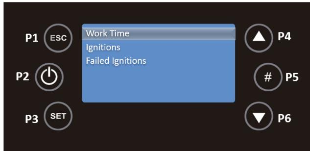
Using the P4 and P6 keys, select the submenu you wish to consult and press P3 to validate. To return to the Service menu, press P1.
