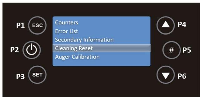
In this function you can switch this function on or off. To return to the Service menu, press P1.
