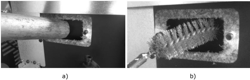
Figure 144 – Example K300, K400 a) Aspirate the interior; b) Cleaning with a brush
