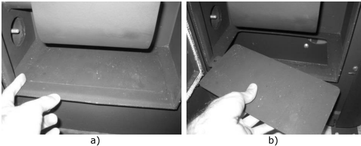
Figure 140 – Cleaning the Pellet Fire Unit's interior
