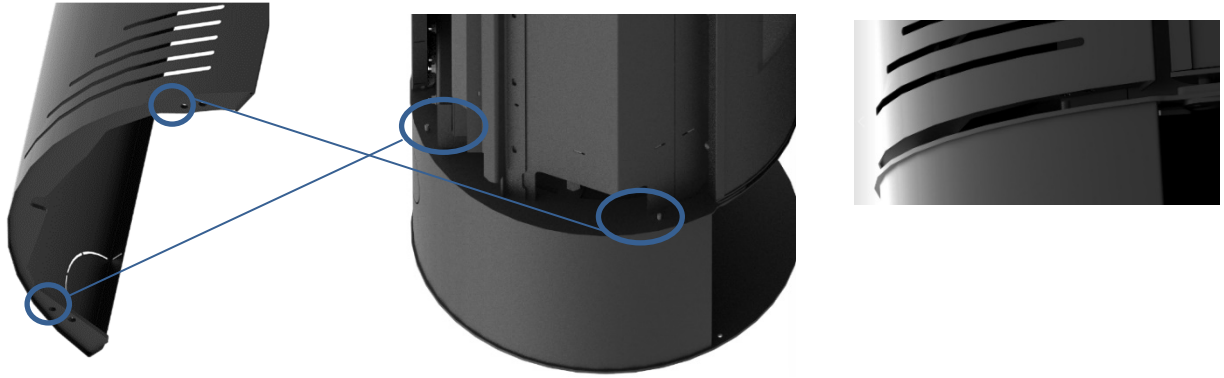
Figure 18 - Centering of the side casing with the equipment
