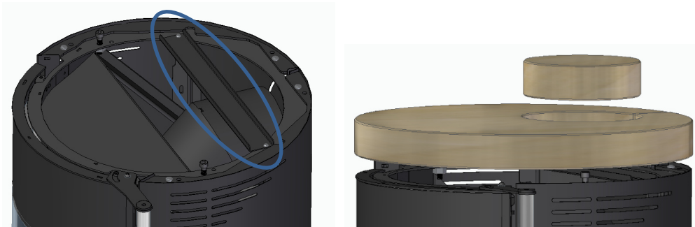
Figure 14 - Placing the top cover on the equipment with horizontal smoke outlet
