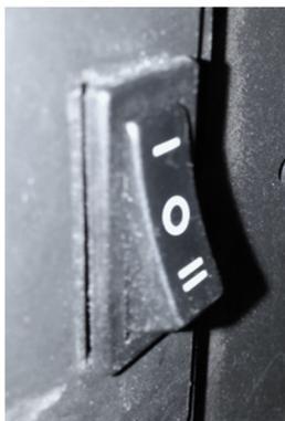
**Position I** – Tangential fan automatically turns on with an air flow of 60m<sup>3</sup>/h when the thermostat reaches 50 °C.
