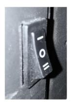
**Position I** – Tangential fan automatically turns on with an air flow of 60m3/h when the thermostat reaches 50 °C.
