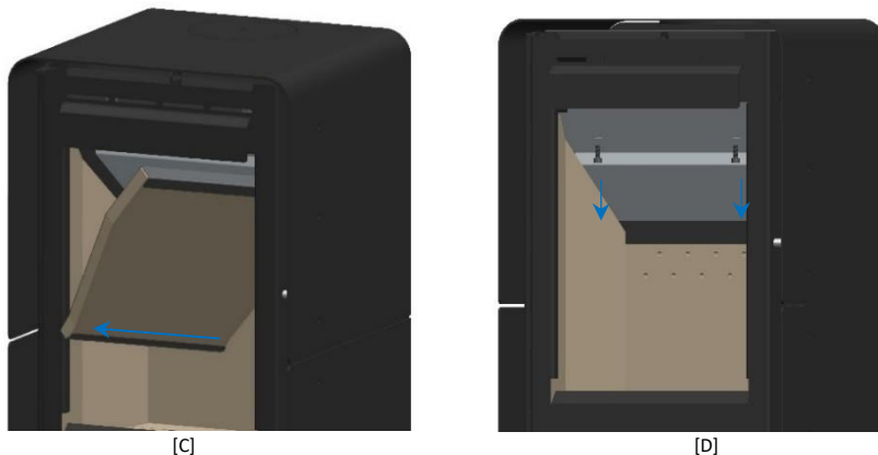
Figure 44 – Sequence that must be followed to remove the fume baffle (except M12F Eco and M20 Eco)
