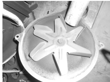
Figure 116 - a) Vacuum the extractor cover; b) Vacuum the extractor
