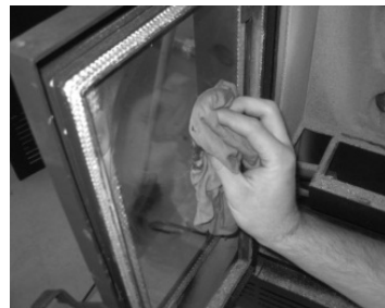
Figure 103 - Cleaning the glass: a) moisten a soft cloth with liquid; b) clean the glass with the cloth
