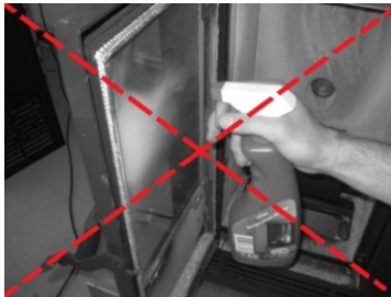
Figure 102 - Incorrect cleaning of the glass
