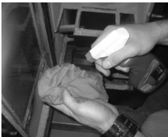
Figure 103 - Cleaning the glass: a) moisten a soft cloth with liquid; b) clean the glass with the cloth
