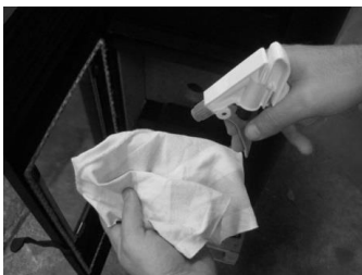
Figure 63 - Cleaning the glass: Applying liquid to the cloth
