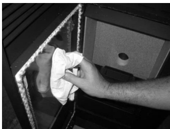
Figure 64 - Cleaning the glass: Cleaning the glass with the cloth
