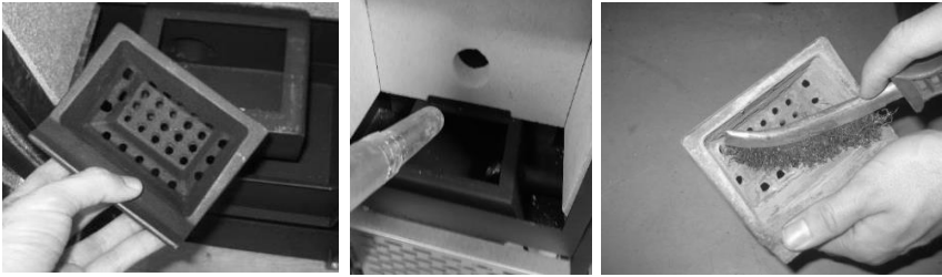
a) Burner removal
