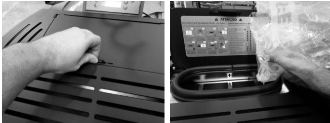
Figure 18 – Refueling the pellet tank
