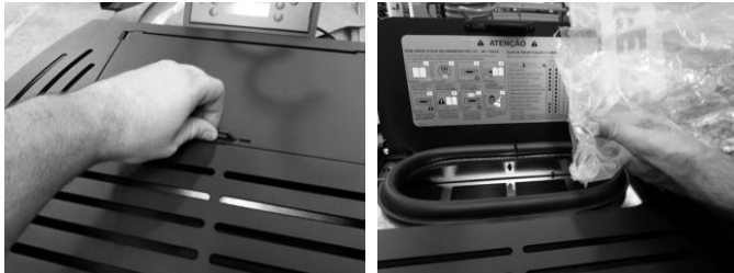
Figure 18 – Refueling the pellet tank
