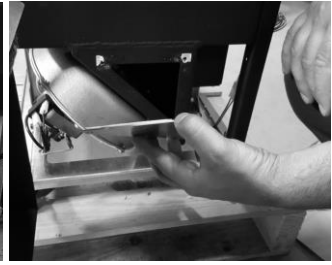
c) Frontal opening smoke path
