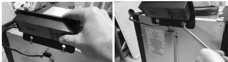
Figure 17 – Fixation du display
