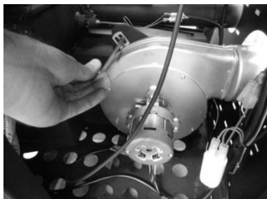
Figure 42 - a) Remove the screws; b) Remove the extractor
