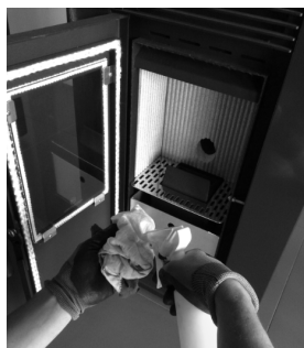
Figure 45 - Cleaning of the glass: a) moisten a soft cloth with liquid; b) clean the glass with the cloth
