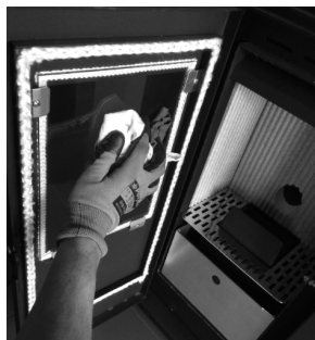
Figure 45 - Cleaning of the glass: a) moisten a soft cloth with liquid; b) clean the glass with the cloth
