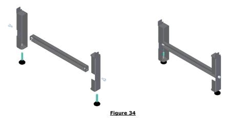
To tighten the 2 screws DIN 912 M10x20mm you will have to use the Allen key n<sup>o</sup>6 the process is very similar to the previous step, but in this case you will have to place the front and rear rails (the longest ones) between the vertical columns and the side beam. Tighten the screws but do not tighten them to allow the subassembly to fit the equipment.
