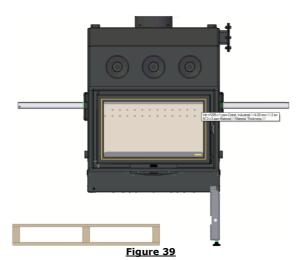
Place the second subassembly in the position you can see in the following image, use the other 2 screws removed earlier (DIN 6921 M6x20mm) to attach the subassembly to the equipment. Pay special attention to the position of the front and rear rails, as you can see in the image below, they should be inside the vertical columns of the subassembly. If you do not, you won't be able to put them in their place afterwards.
