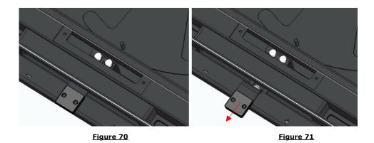
→ Remove the combustion control by pulling it up and then pulling it out through the door. Be careful when removing it, as several fiberglass cords are glued to the bottom of the control to ensure that the joints between the parts are watertight.
