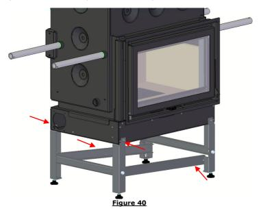
Remove the screws and the side member from the first sub-assembly, put the front and rear limbs in place and replace, this time within the front and rear limbs, the lateral limb. Fix it again with the screws. Before tightening all the screws well, carefully check the position of all the parts for maximum perpendicular to each other.
