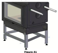
With the machine in its final position, perform the leveling using the 4 feet of leveling and a level that we recommend to place on the door rim to level the left right position and inside the combustion chamber to level the front and back. Remember to check again when you have finished both positions, as changing one level may affect the other.
