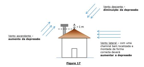
The depression differences caused by the outside wind are also felt inside the house and the placement of stoves in the area directly exposed to the wind can increase the depression created in the chimney, a fact that competes with the pressure caused by the wind outside the house, which works in an inversely proportional way, that is, the zone of lower depression will be the area directly exposed to the wind.
