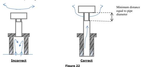
The dome of the chimney shall allow good air circulation and shall be placed at least 1 m above the summit or any other obstacle less than 3 m away; If you need to increase the circulation you should increase the height of the chimney.
