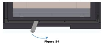
From the central point of the control to the rightmost position, the primary air is progressively opened while the secondary air remains 100% open in this zone.
