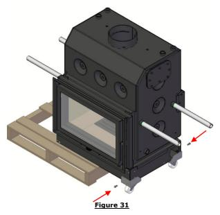
Move the equipment over the pallet, leaving the left front corner in the air, as shown in the image. Place the wheel and fix it with the screw, as was done with the previous wheels.
