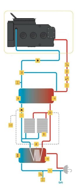
Scheme 3 – Installation for central heating (AC) and Sanitary Hot Water (ACS) with solar panel
