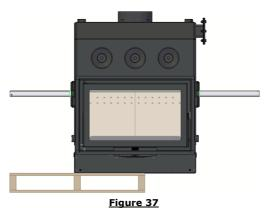
Tilt the equipment using the transport bars, to gain the necessary space and place the first subset that we have assembled. Fix the subassembly by placing two of the screws we removed earlier (DIN 6921 M6x20mm) and secure them tightly.
