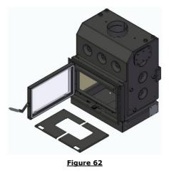
→ Remove the 2 vermiculite plates from the back of the chamber, to remove these plates first move them upwards about 10mm and then pull the bottom towards the door so that it rotates at its top, then let it go down so that it is free of the plate that fixed it. Remove the plate and repeat the operation with the other plate later.
