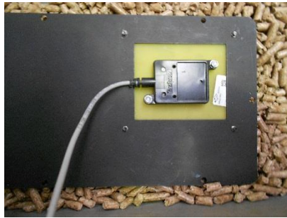
Figure 26 – Placement of the sensor over the pellets
