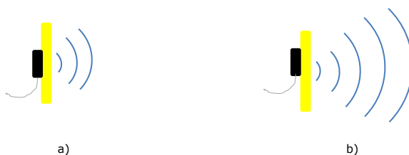
Figure 2 – Difference between a level sensor with low sensitivity (a) and high sensitivity one (b)
