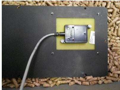
Figure 6 – Placement of the sensor over the pellets
