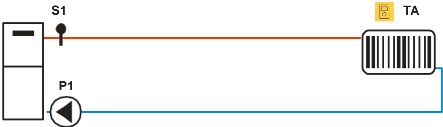
Figure 49 - Simple connection only the central heating radiators
