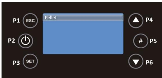
With the P4 and P6 keys you can change the system's combustion power. Press the P3 key to save your changes and use P1 to go back.
