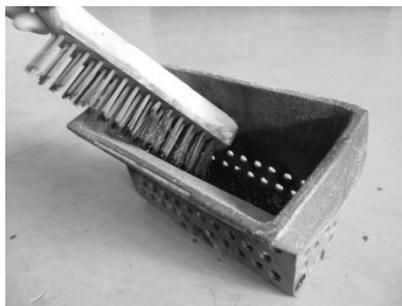
**Figure 31 - Firing basket cleaning**
