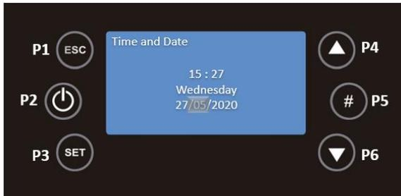
The Year follows the same procedure, press the P4 and P6 keys to move to the Year, use the P3 key to edit this field, the year will appear in editable mode. With P4 and P6 select the desired year and press P3 to validate.
