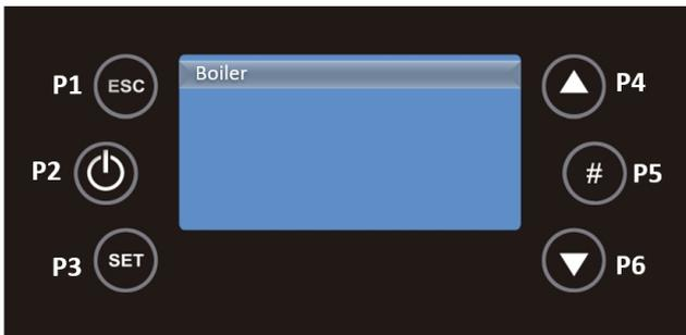
This submenu allows you to change the value of the Compact thermostat, with the P4 and P6 keys. The minimum and maximum values can be programmed.
