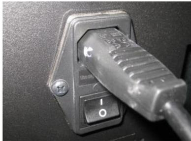
Figure 12 - Power connection plug
