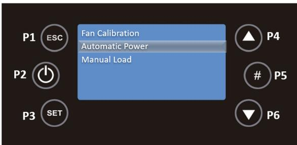
In this submenu you can set the firing power only in automatic mode. If you set it, all power change menus will not be visible. With P4 and P6 you must select On or OFF and validate your choice with the P3 key.
