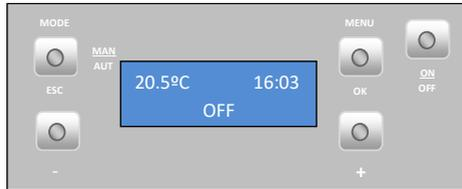
**"Auto" mode:** in this mode, the unit will be turned on at maximum power until reaching a temperature of 1°C above the selected temperature (set point temperature). Upon reaching the set temperature, the unit toggles to the minimum operating power.
