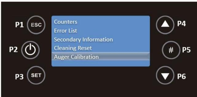
In this sub-menu with the keys P4 and P6 you can adjust the amount of pellets to be fed, between -7 (-14%) and 7 (+14%). To return to the Service menu press P1.
