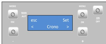
To **activate the timer mode** press "set". The display starts to flash. Press the "+" or "-" key to select "On" or "Off" and then "ok" to confirm. Press the "+" key to go
