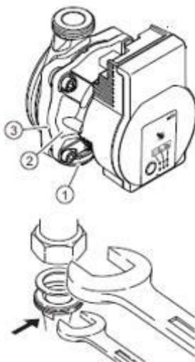
**Figure 50 - Pump installation**
