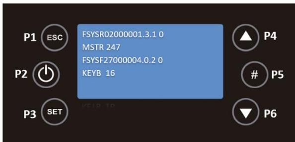
To return to the Keypad menu, press P1. Pressing this key twice brings up the menus Settings, Keypad, Service and System Menu.
