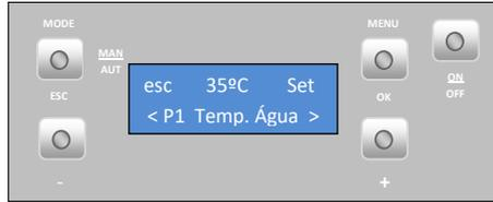
To set the **operating power** (1 to 5) for Programme P1, press "set". The display starts to flash. Press the "+" or "-" key to select the desired power and then "ok" to confirm. Press the "+" key to go to the "P1 Dia" (P1 Day) menu.
