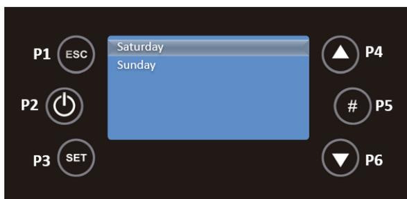
You should press P3 and this field will be in editable mode, flashing. Press P4 and P6 to select the desired time and then use the P3 key to save. You must repeat this process for the time at which the equipment should shut down, with the P4 and P6 keys. Finally you must captivate the interval with the P5 key, and a check mark will appear on the right side of the interval.
