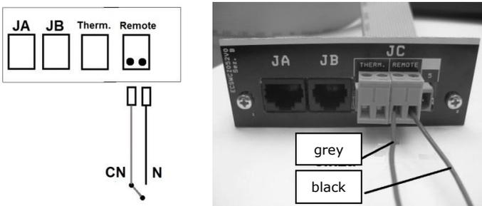
**Figure 21 - Wired external control connections**
