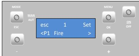
To select the **days of the week** that you want the P1 Programme to run, press "set" and then select the day of the week using the "-" and "+" keys. Press "set". The display starts to flash. Select "On" or "Off" using the "-" and "+" keys. Press "ok" to confirm the selection. Press the "esc" key to go to the "P1 Dia" (P1 Day) menu. Press "esc" twice and then "+" to go to the "ConFigureções" (ConFiguretion) menu.
