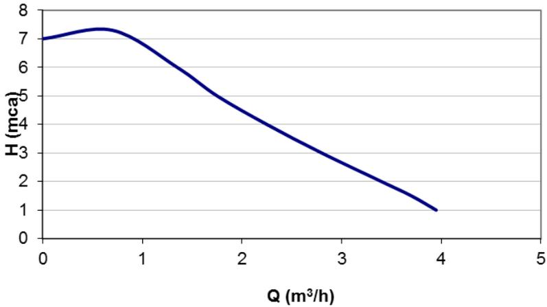
Figure 45 – Circulating pump performance graph
