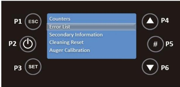
This submenu shows the last 10 errors that occurred, on each line the error code and the date and time when it occurred are shown. To return to the Service menu, press P1.
