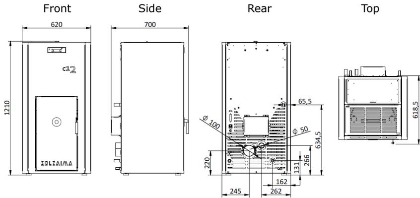
**Figure 2 – Compact pellet Compacta Eco 12 dimensions**
