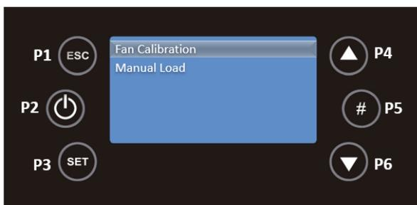
In this submenu with the keys P4 and P6 you can adjust the fan speed, between -7 (-21%) and 7 (+21%). To return to the Service menu press P1.
