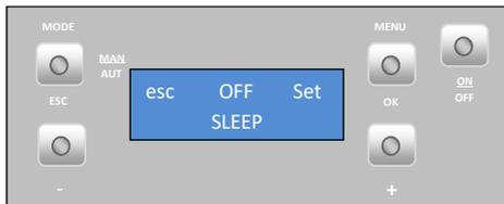
Press "set". The display starts to flash. Select the desired time using the "-" and "+" keys. After choosing the time, press "ok" to confirm. Press "esc" to return to the menu and then "+" to go to the conFIGuration menu.
