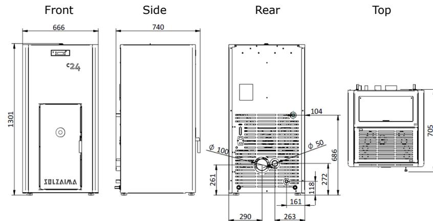
**Figure 4 – Compact pellet Compacta Eco 24 dimensions**
