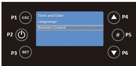
With the P4 and P6 keys you can activate or deactivate the Remote Control, pressing P3 to validate the action.
