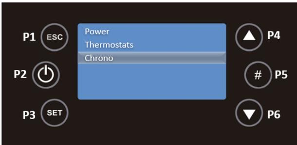
Then you must enter the Program submenu, using the P6 key to select and P3 to validate the choice.
