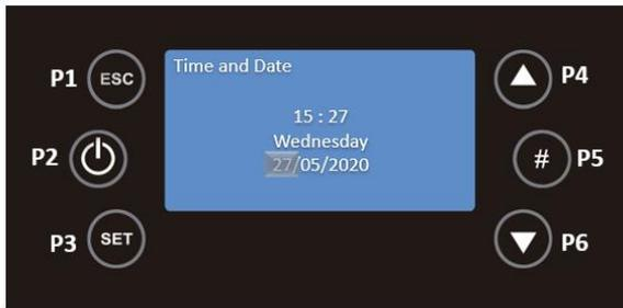
To edit the Month you must use the P4 and P6 keys to select this field and then P3, the month will appear in editable mode, with P4 and P6 select the desired month and press P3 again to validate.
