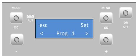
Press "set" again and, when the display starts to flash, press "+" or "-" to select "On" or "Off". Press "ok" to confirm the selection. Press the "+" key to go to the "P1 A. Inicio" (P1 A. Start) menu.
