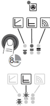
**Figure 54 - Lock/unlock the button**
