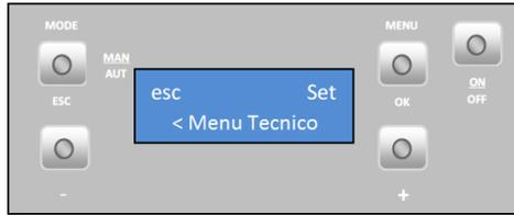
Press "Ok"; the letter "A" starts to flash. Using the "+" and "-" keys, select the desired letter. Press "Ok" to confirm; the numbers "00" start to flash. Using the "+" and "-" keys, select the desired number. Confirm by pressing "OK" to go to the "ConFigureção" ("Settings") menu.
