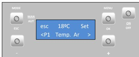
To set the **water set point temperature** (only for the **back compact model**) for Programme P1, press "set". The display starts to flash. Press the "+" or "-" key to
