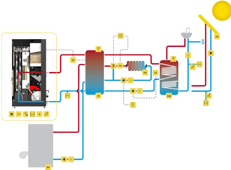
**Figure 40 - Connection to underfloor heating, combined with another backup compact and sanitary water combined with solar panel**
