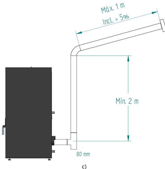
**Figure 10 - Examples of type installations**
