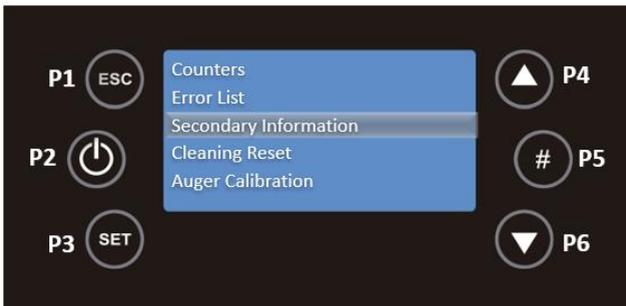
In this function you can query the product code, the status of the fume extractor, the worm, the ambient fan, and the status of the outputs.
