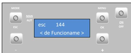
This menu indicates how many working hours the compact has after the last service. Number of hours the service should take place.
