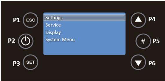
Select the Language submenu with the P6 key and to validate the entry in this submenu the P3 key.
