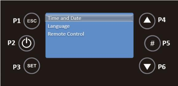
Now in the Date and Time menu, select Time, with the P4 and P6 keys, and press the P3 key, the time will appear in editable mode, flashing, with P4 and P6 select the correct time and press P3 to validate.
