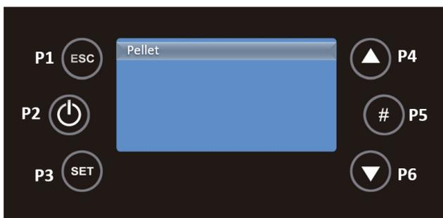
With the P4 and P6 keys you can modify the combustion power of the system. Press the P3 key to save your changes and use P1 to go back.
