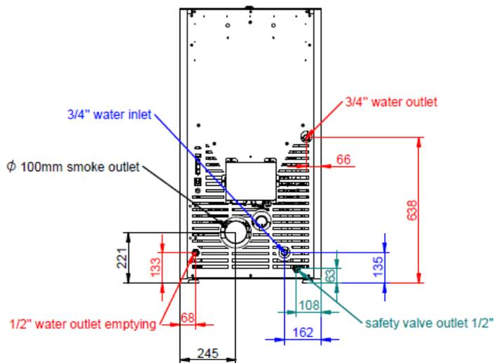
**Figure 5 - Hydraulic connections for the Compacta Eco 12 compact**
