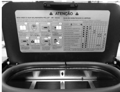
Figure 23 - Label with maintenance tasks
