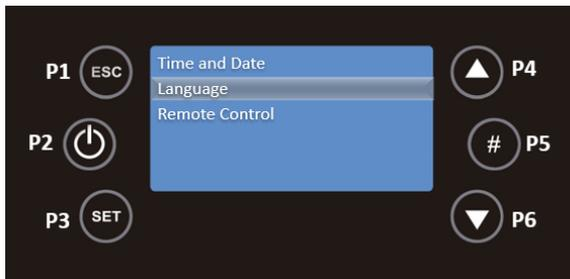
Within this submenu, with P4 and P6 select the desired language and press the P3 key again to validate.
