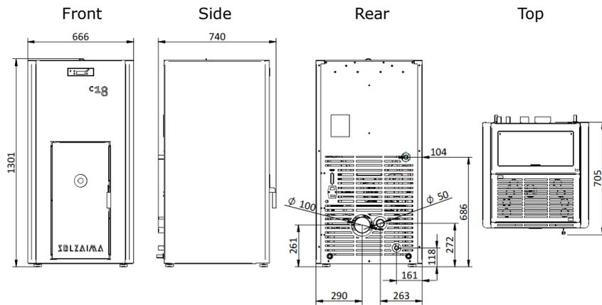
**Figure 3 – Compact pellet Compacta Eco 18 dimensions**
