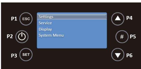
With the P6 key select the Remote Control submenu and to validate the entry in this submenu the P3 key.
