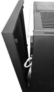
Figure 16 – Removing the side covers
