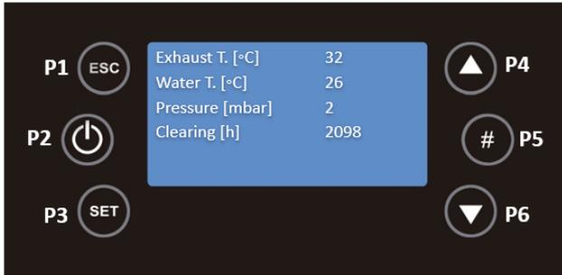
With the P4 and P6 keys you can scroll through the different variables. The values displayed are the values measured On-Line.
