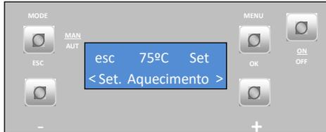
**Note:** in the water equipment, the water temperature can be regulated by the user (water set-point temperature) between 50 and 80°C.
