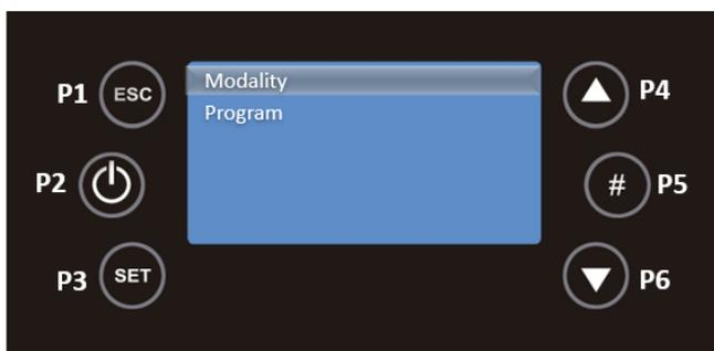
By selecting Mode with the P3 key you can select which chrono mode you want. Use the P4 and P6 keys to select between Daily, Weekly, or Weekend, use the P2 key to activate/deactivate the choice, and P3 to save the changes.
