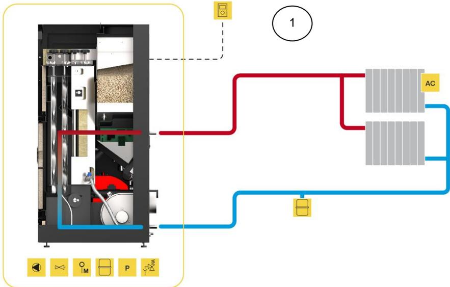
**Figure 36 - Simple connection to central heating radiators only**
