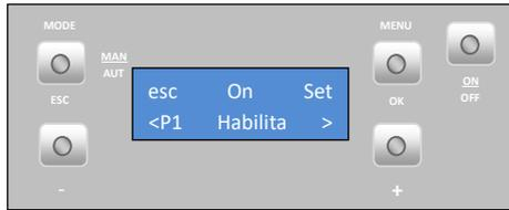
To set the **starting time** for Programme 1, press "set". The display starts to flash. Press the "+" or "-" key to select the desired time and then "ok" to confirm. Press the "+" key to go to the "P1 H. Stop" (P1 Time Stop) menu.
