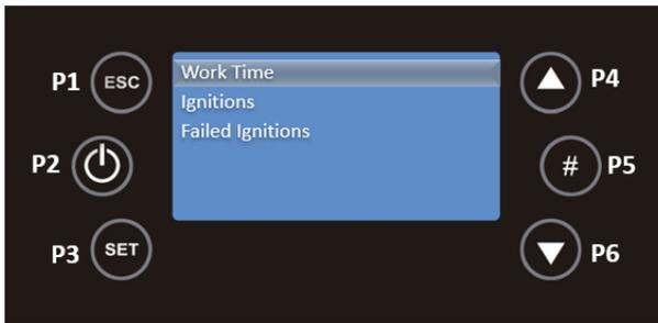
With the P4 and P6 keys, select the submenu you wish to consult and press P3 to validate. To return to the Service menu, press P1.
