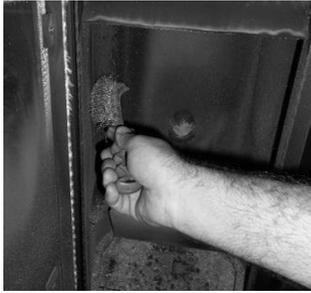
**Figure 29 - Cleaning the inside of the water compact**
