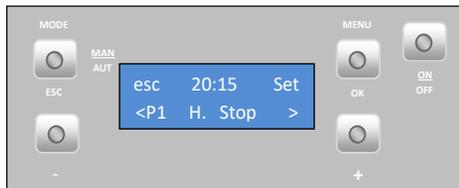
To set the **set point room temperature** for Programme P1, press "set". The display starts to flash. Press the "+" or "-" key to select the desired temperature and then "ok" to confirm. Press the "+" key to go to the "P1 Temp. Água" (P1 Water Temp) menu.
