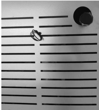
**Figure 13 – Ambient Temperature Probe**
