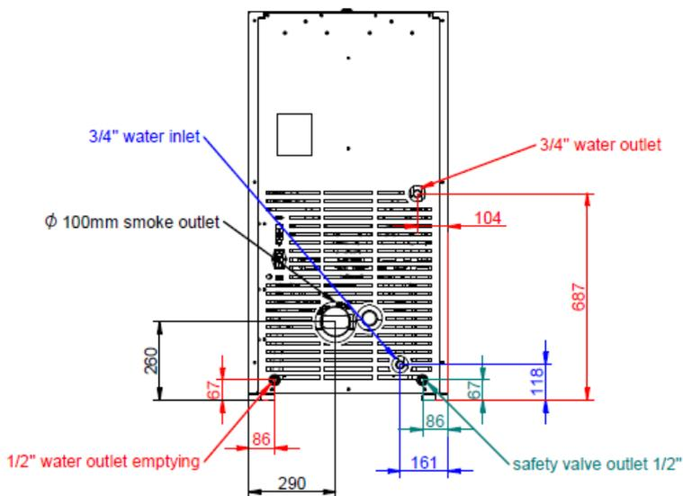
**Figure 6 - Hydraulic connections for the Compacta Eco 18 and 24 compacts**
