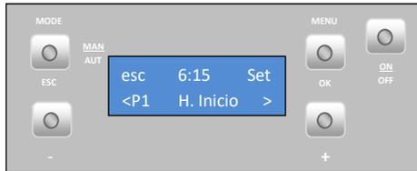
To set the **stopping time** for Programme 1, press "set". The display starts to flash. Press the "+" or "-" key to select the desired time and then "ok" to confirm. Press the "+" key to go to the "P1 Temp. Ar" (P1 Air Temp) menu.
