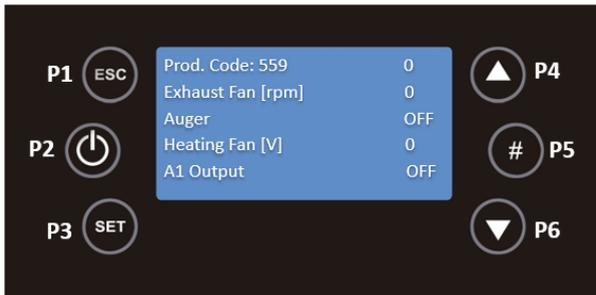
It is possible to query the fume temperature, room temperature and the state of the inputs. Whether the state of the input is open (0) or closed (1).
