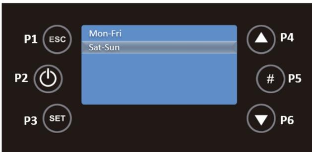
You should press P3 and this field will be in editable mode, flashing. Press P4 and P6 to select the desired time and then use the P3 key to save. You must repeat this process for the time at which the equipment is to turn off, with the P4 and P6 keys. Finally you must activate the interval with the P5 key, and a check mark will appear on the right side of the interval.
