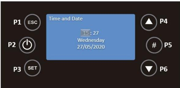
The same must be done for Minutes, with P6 select Minutes and press P3, the minutes will appear in editable mode, flashing, with P4 and P6 select the correct minutes and press P3 to validate.
