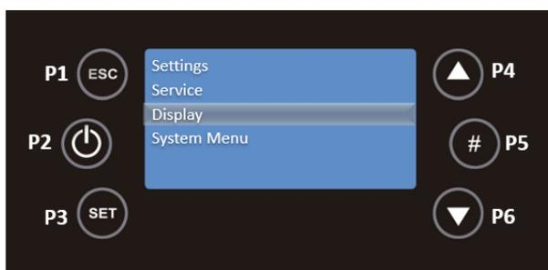
In this menu there are the functions Contrast, Min Brightness, Screen Saver and Firmware Codes.
